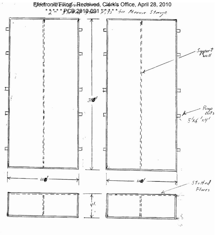
All walls are power concret All slotled floors are precast concrete
